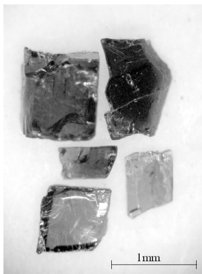
Figure 4. Single crystals of the HP VOPO obtained by cooling the melt from 1200 to 600° over 60 h at 3 GPa.
